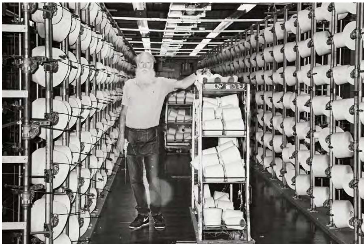
George Westmoreland, known as "Red", loads yarn packages in the creel of a modern day warper at White Oak Mill.
