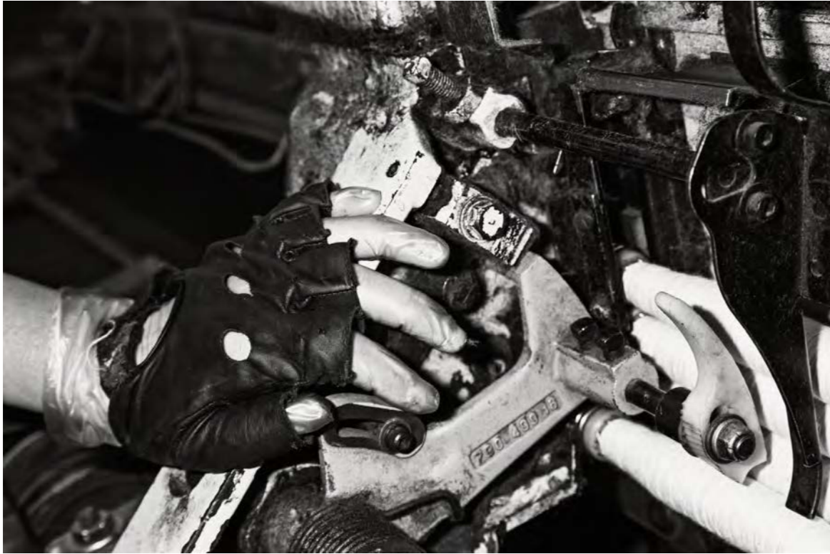
Loom technician checks the setting on the bobbin transfer of the X3 shuttle loom which inserts the weft yarns.
