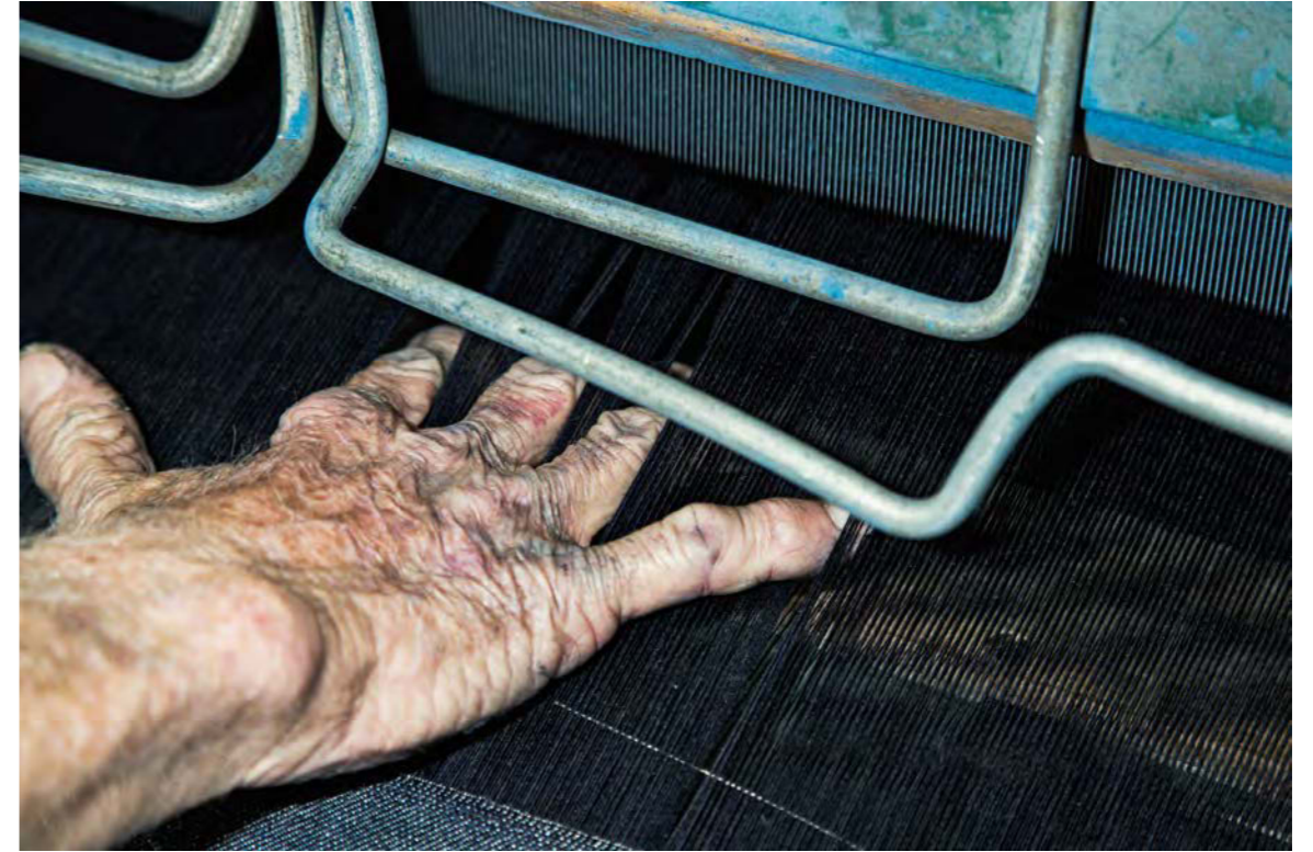
Experienced hands feel the warp to check for tension and harness heights.
