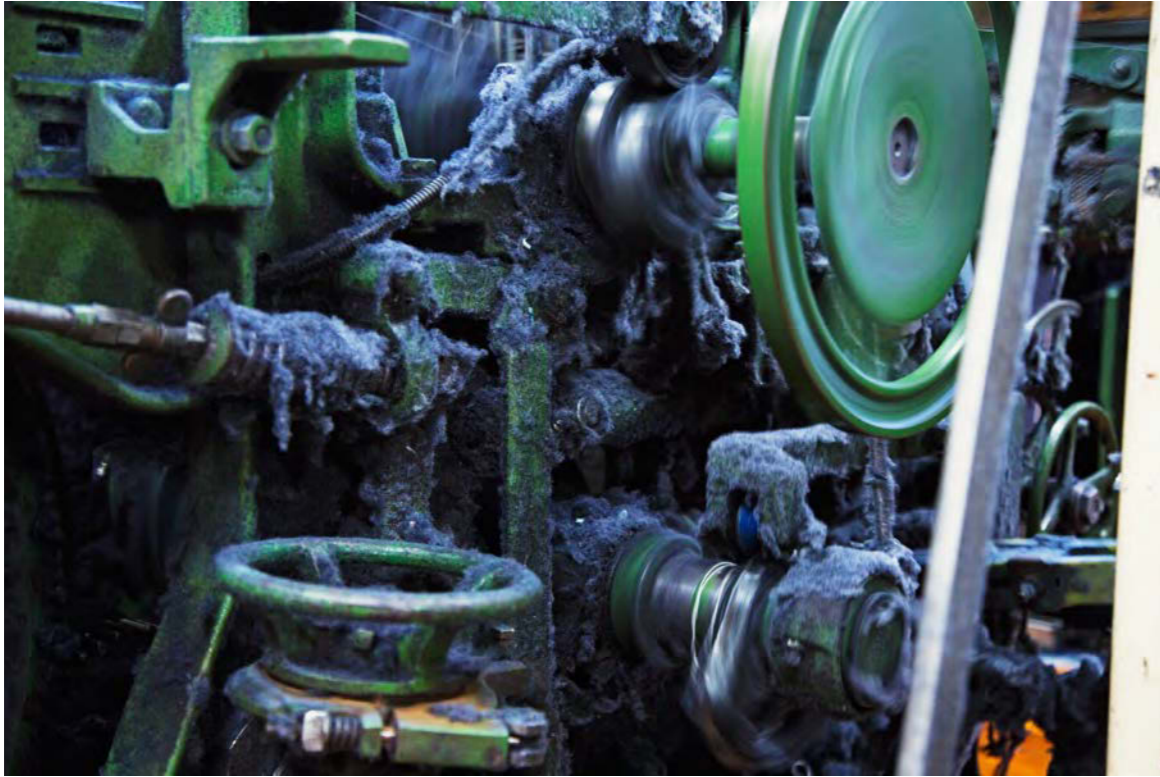
The gears and pulleys of the X3 shuttle looms, c. 1940s, work in rhythm to weave vintage selvage denim.
