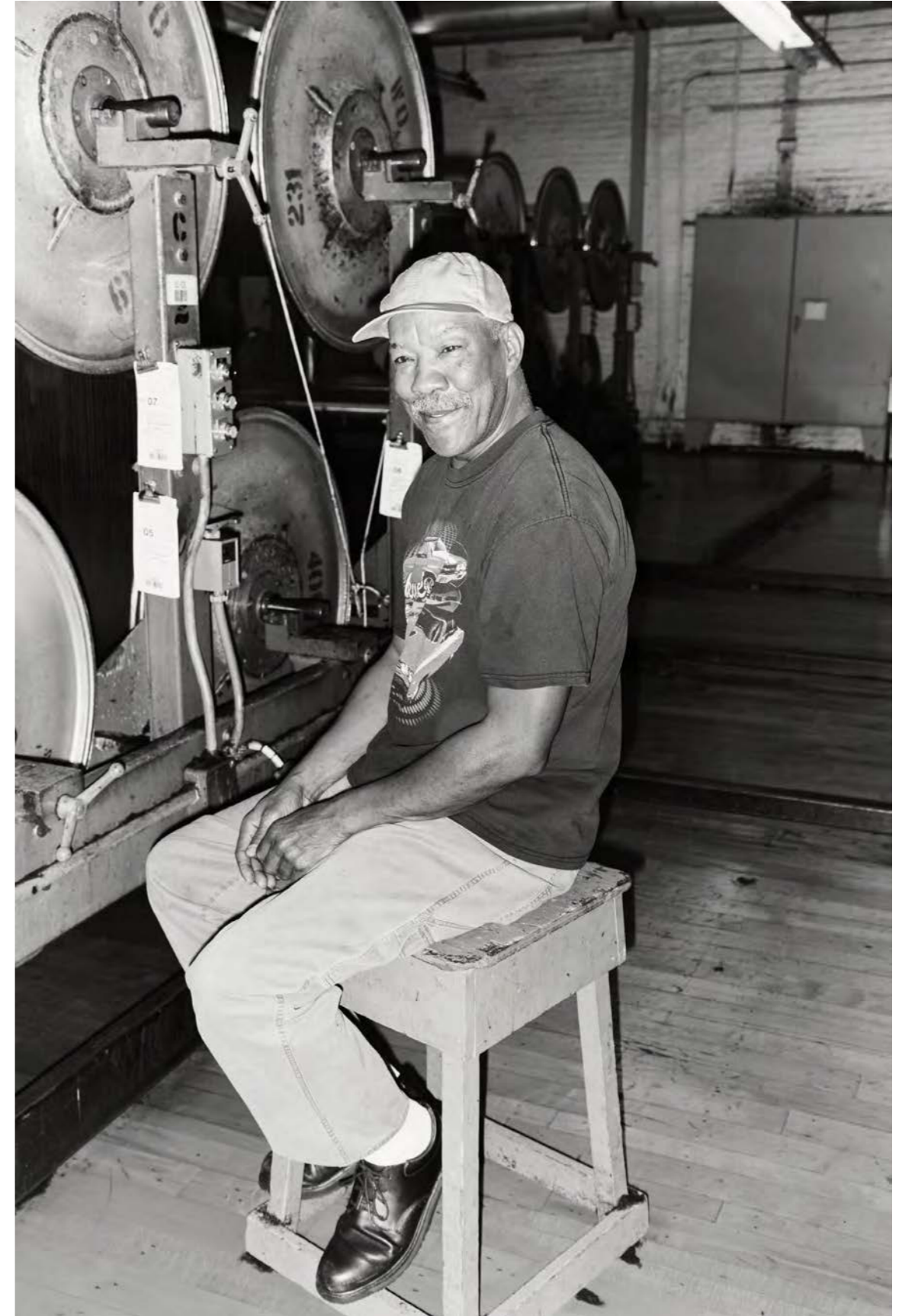
Slasher Operator Jerome Arnold monitors creeling area of slasher where section beams are combined to prepare the warp for weaving.
